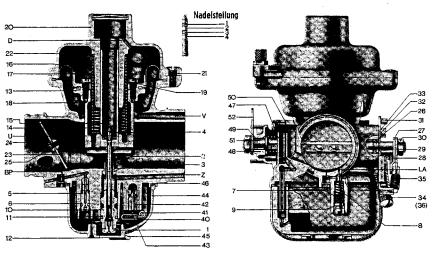
next notch in the jet needle. If the needle is suspended higher up, this will result in a richer mixture and vice versa.
