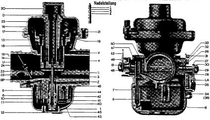
set in such a way that the float top edges are parallel to the top edge of the float chamber.
