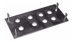
mounting tabs will fit down over the screws. Nuts can be tightened down to secure it. For a composite aircraft installation, the bottom of the plate (shown above) should be floxed and the holes in the plate filled with flox before applying fiberglass layers over it to secure it to the fiberglass structure.
